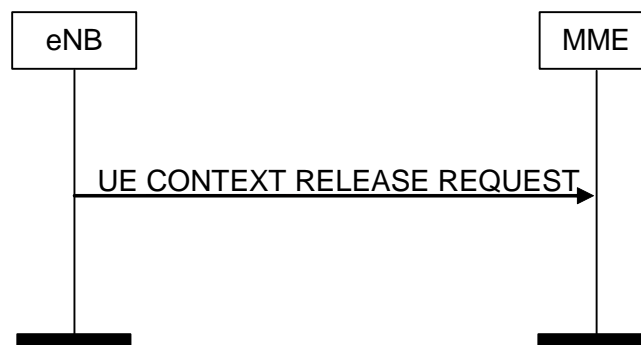
Figure 8.3.2.2-1: UE Context Release Request procedure. Successful operation.
