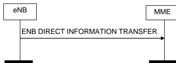
Figure 8.13.1.2-1: ENB Direct Information Transfer procedure. Successful operation.
