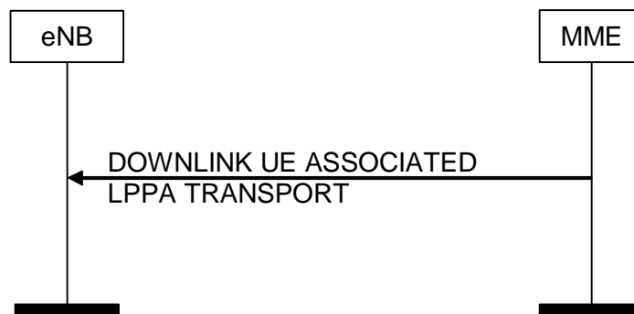
Figure 8.17.2.1-1: DOWNLINK UE ASSOCIATED LPPA Transport Procedure
