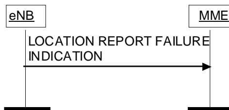
Figure 8.11.2.2-1: Location Report Failure Indication procedure.
