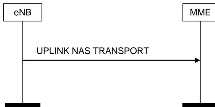
Figure 8.6.2.3-1: UPLINK NAS TRANSPORT Procedure
