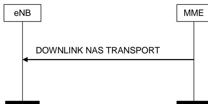
Figure 8.6.2.2-1: DOWNLINK NAS Transport Procedure
