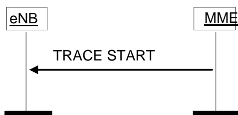
Figure 8.10.1.2-1: Trace Start procedure.
