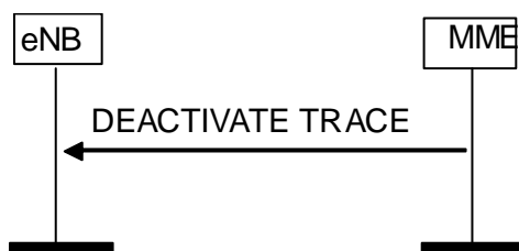
Figure 8.10.3.2-1: Deactivate Trace procedure. Successful operation.
