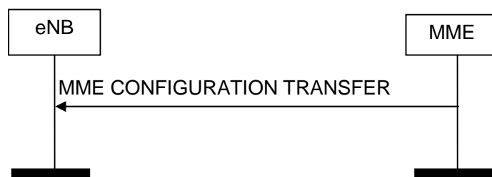
Figure 8.16.2.1-1: MME Configuration Transfer procedure. Successful operation.
