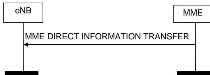
Figure 8.14.1.2-1: MME Direct Information Transfer procedure. Successful operation.
