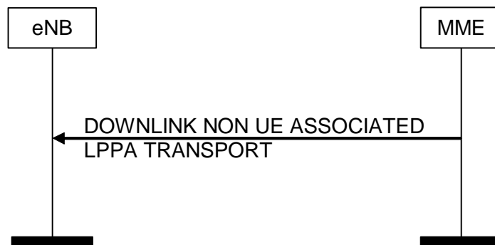
Figure 8.17.2.3-1: DOWNLINK NON UE ASSOCIATED LPPA Transport Procedure
