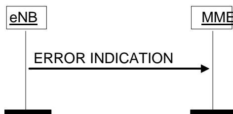
Figure 8.7.2.2-2: Error Indication procedure, eNB originated. Successful operation.
