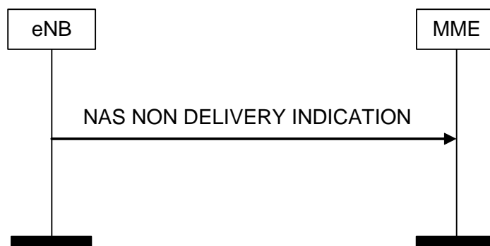
Figure 8.6.2.4-1: NAS NON DELIVERY INDICATION Procedure
