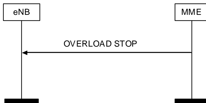
Figure 8.7.7.2.-1: Overload Stop procedure
