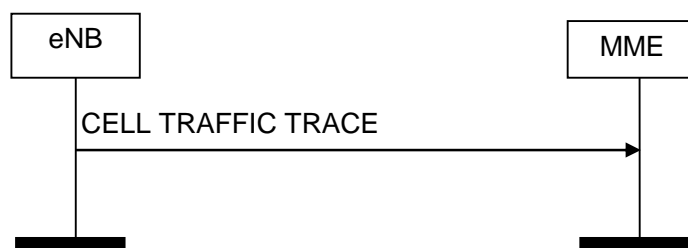
Figure 8.10.4.2-1: Cell Traffic Trace procedure. Successful operation.
