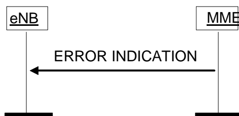
Figure 8.7.2.2-1: Error Indication procedure, MME originated. Successful operation.
