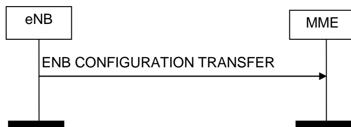
Figure 8.15.2.1-1: eNB Configuration Transfer procedure. Successful operation.
