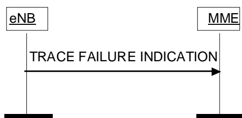
Figure 8.10.2.2-1: Trace Failure Indication procedure.
