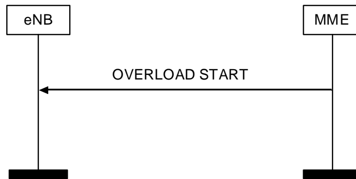
Figure 8.7.6.2-1: Overload Start procedure
