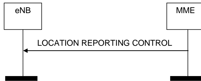
Figure 8.11.1.2-1: Location Reporting Control procedure. Successful operation.
