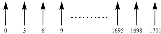
Figure 244—Basic structure of DL preamble, 2048-FFT
