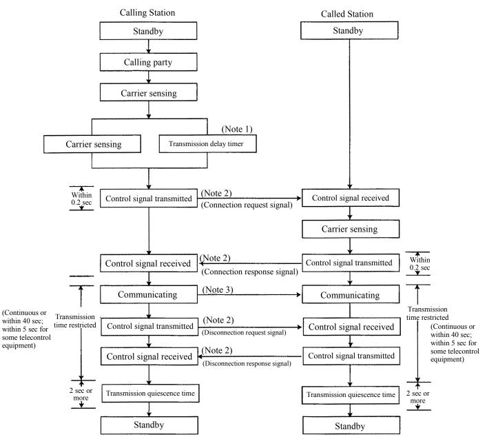
Figure 3.4 Example of the Channel Connection Procedure in Semi-duplex and Duplex Operation (Fixed and Manual Channel Switching)
