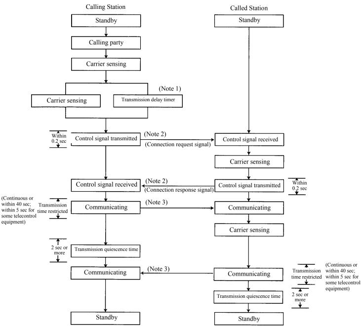
Figure 3.2 Example of the Channel Connection Procedure in a Simplex Operation (Fixed and Manual Channel Switching)
