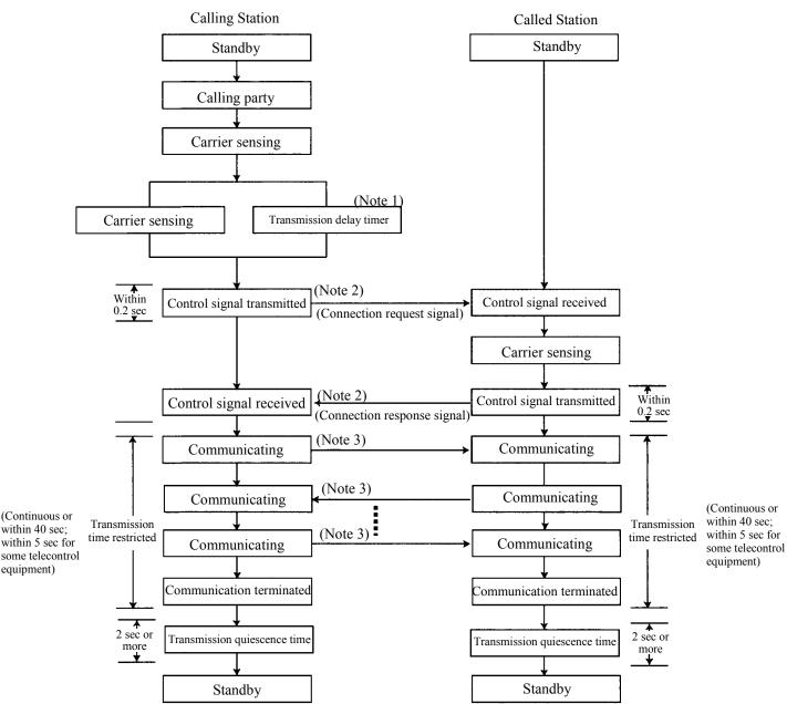
Figure 3.3 Example of the Channel Connection Procedure in a Simplex Operation (Fixed and Manual Channel Switching)
