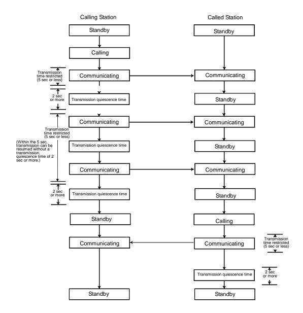
Figure 3.1 Sample Transmission Times in a Simplex Operation (426MHz Band Telecontrol with Including the Data Transmission Annexed Thereto)
