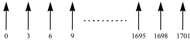
Figure 244—Basic structure of DL preamble, 2048-FFT
